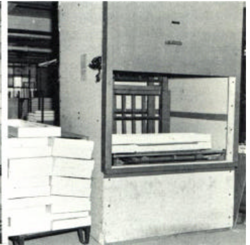
Prefab enclosure, automatic doors, safety devices meet rigid state safety code for lamp manufacturer.
