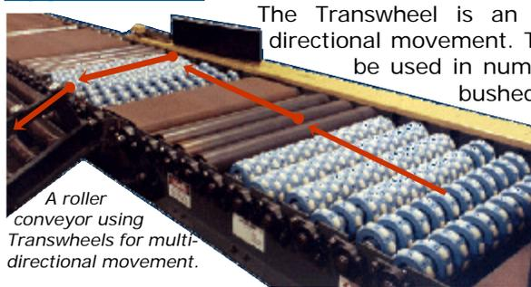
*A roller conveyor using Transwheels for multi-directional movement.*
