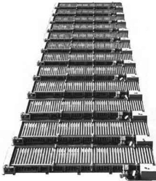
Pallet load accumulators speed load transfer and accomodate 5° ship roll
