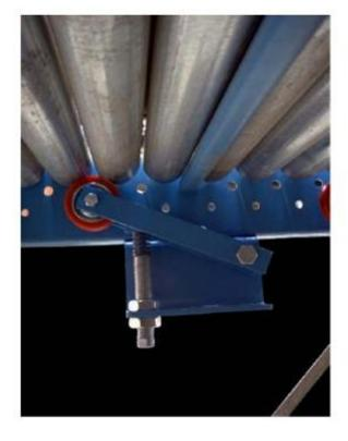
rolls over the two Rollerslo's®, the Palletflo® wheel starts to turn, the hysteresis effect absorbs the energy of the turning rollers and reduces its speed. The elastomer hysteresis effect of the Palletflo® wheel acts as a brake and slows the flow of the object moving down the conveyor.
