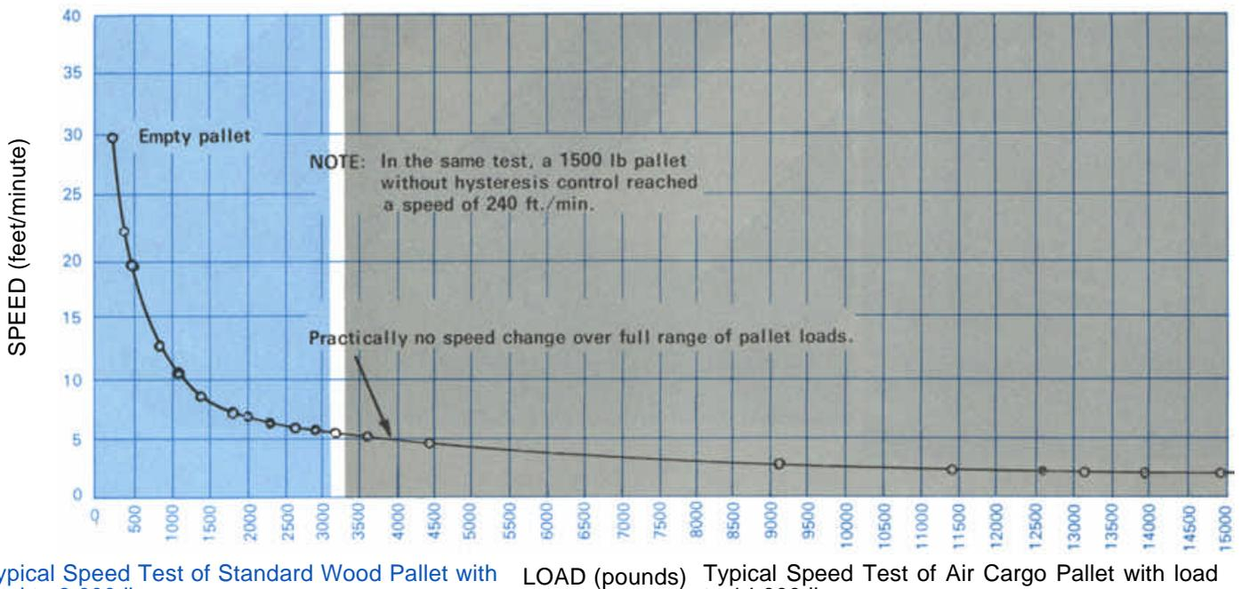
Typical Speed Test of Standard Wood Pallet with load to 3,000 lbs.
