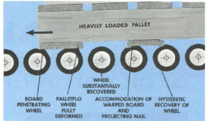
Palletflo wheels deform to accommodate any standard pallet. Hysteresis in each controls pallet speed.
