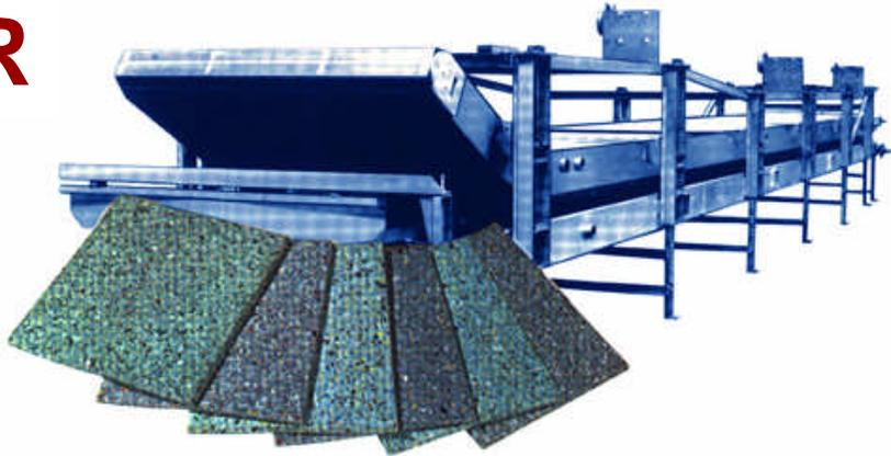
Rebonder can produce carpet cushion in a continuous 72" width sheet, with controlled thicknesses from 1/4" to 1" and at speeds from 10' to 60' per minute. The 200 foot long Rebonder has a production potential of 19,000 square yards per eight-hour shift.
