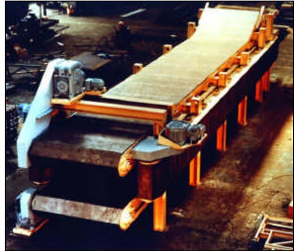
In this system, scrap foam is shredded, mixed evenly with bonding agents, compressed, cured, rolled up and packaged ready for shipment – in an uninterrupted production process. The finished underlayment can be of foam only or with scrim bonded to one or both sides. Its quality is exceptional, the bonding tight and the thickness predictably uniform, with a pleasing distribution of the various colors of scrap foam.
