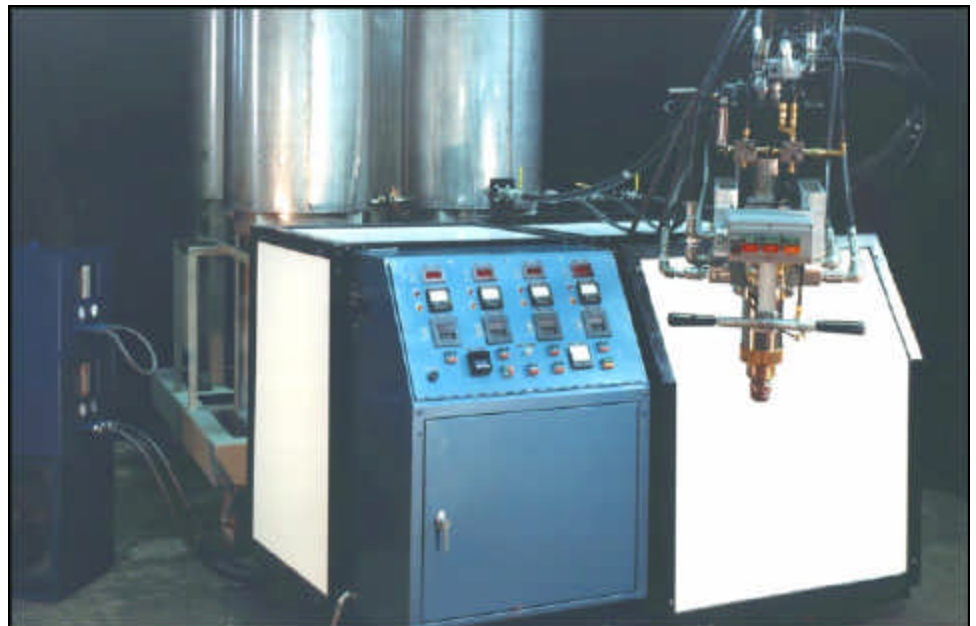
"User friendly" control panel - Regulates and displays temperature, pressure and flow of resin, catalyst, additive and blowing agent - Incorporates shot time and mixer speed control - Stainless steel day tanks (added as an optional feature) - provide chemical temperature control
