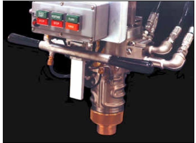
Mixing head temperature control system reduces premature frothing and foaming. Wrap-around stainless steel cooling jacket permits coolant to maintain favorable phenolic mix temperature for "hot" formulations.
