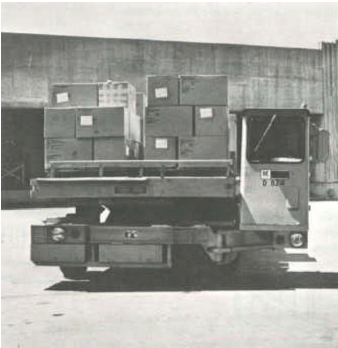
APPROACHING DOCK, driver operates controls to swing his cab aside and to elevate Karry-All cargo deck for perfect line-up with dockside conveyor. He will then lower the cargo restraining bar, clearing the way for unloading.
