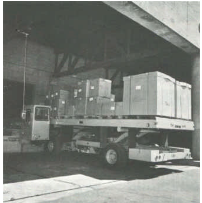
AUTOMATIC UNLOADING in seconds: Karry-All driver starts dock-side conveyor, using controls outside cab window. Powered rollers on Karry-All cargo deck swiftly transfer load. All operations are controlled from the cab.
