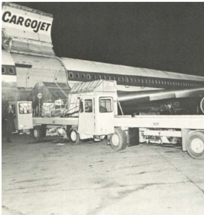
Above, the High-lift Karry-All is used in conjunction with the standard Karry-All. The High-lift remains stationary and provides an elevator loading service—standard Karry-All acts as transport vehicle and also on-off loads the High-lift.
