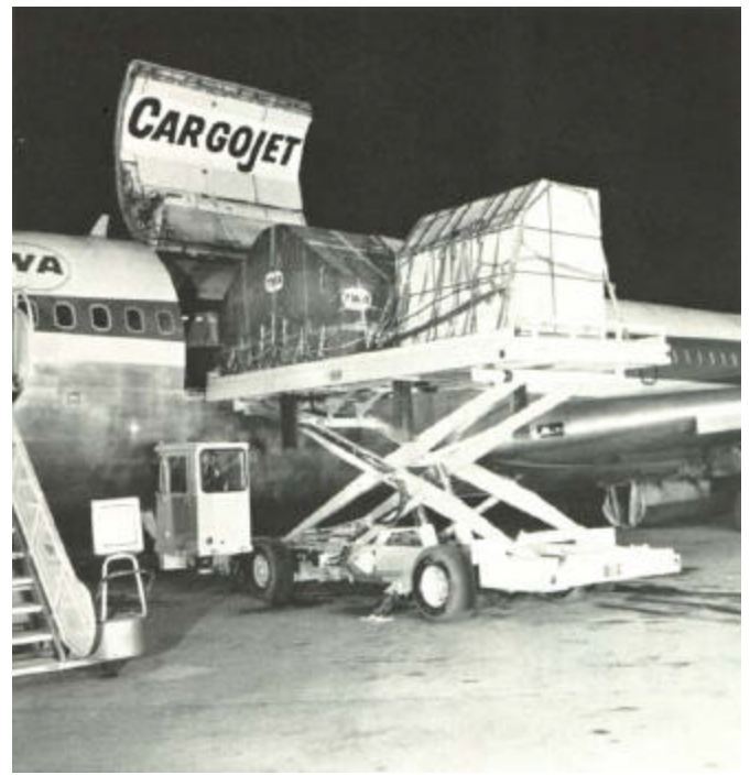
Above, the High-lift Karry-All is being used to transport, elevate, and on-off load. The cargo is loaded automatically, through remote control in little more than one minute per igloo. The High-lift is designed for fast on-off loading.
