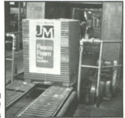
Film wrapped pallet of roofing panels
