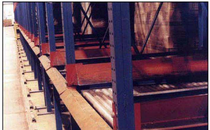
Rollerflo® can handle plastic pallets, wood pallets with very few and or extremely narrow runners as well as a wide variety of sizes and shapes of loads. Rollerflo® conveyors are roller conveyors with a difference! They utilize the hysteresis control principle of Kornylak's patented Palletflo® urethane coated skate wheels.
