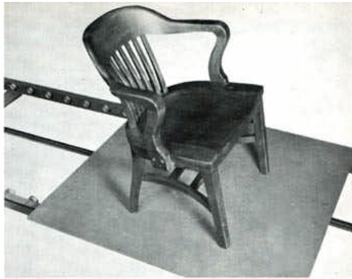
Monoflo permits movement of furniture and other items on pallets in any desired path. Loading, unloading, and stopping for operation can be done at any point.
