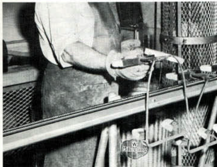
TV picture tube holders are returned to loading end of oven on a Monoflo Conveyor.
