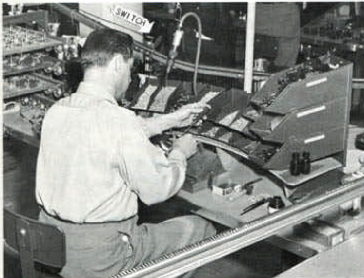
Monoflo in background delivers parts to assembly station where switch automatically stops and starts conveyor as parts are removed. Finished parts are placed on Monoflo in foreground for delivery to next operation.
