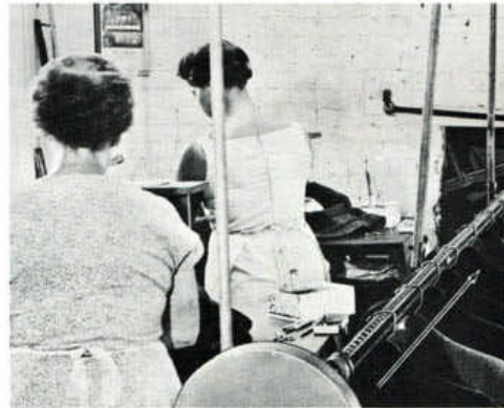
Operators mark buttonholes and place garments on Monoflo Conveyor for delivery to floor below.
